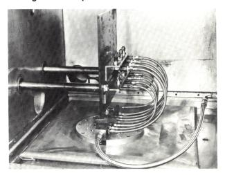
AE246 Hose Assemblies have been thoroughly tested on the test rig shown above under controlled pressure, impulse peaks, temperature and flexing, in order to meet or exceed MIL-H-38360.
