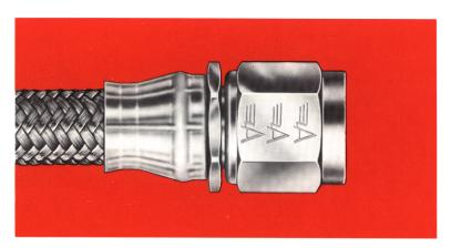
Aeroquip "super-C" fittings provide permanent protection against leakage, even after high temperature aging and impulsing to 250,000 cycles or more. Their reliable performance is due to the independence of the sealing function from the retention function. The service proved "super-C" fittings also feature corrosion resistant materials and reduced envelope dimensions. Its weight saving construction makes it the lightest fitting available in most sizes.
